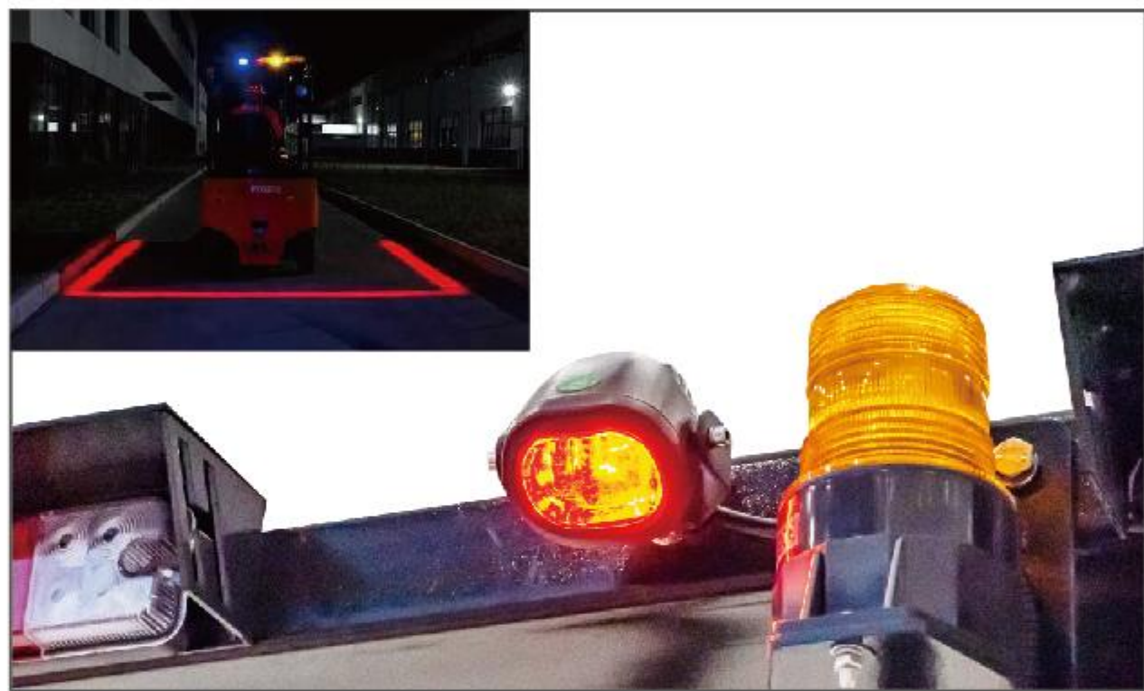
Red Safety Area Lights
